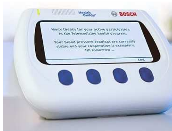
Figure 3.1: Health Buddy, non-video home telemonitoring device
